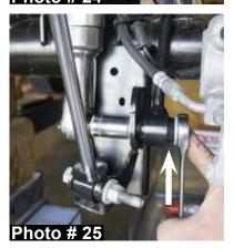
19. Connect the OEM rear track bar to the new Skyjacker rear upper track bar bracket using the OEM hardware & a 21mm socket / wrench. (See Photo # 26) **Note:** Install the OEM bolt with the threads towards the rear of the vehicle.
